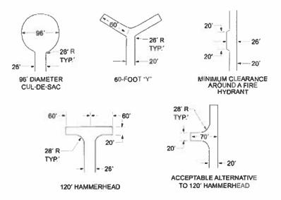
5. Turning Radius: The minimum turning radius for fire apparatus access roads shall be determined by the Fire Code Official.
